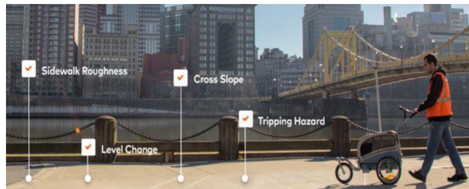
The pathMet© allows a technician to measure slope, contour, surface texture, elevation/level changes and deviation, tripping hazards and other factors that might entail ambulatory obstructions for the handicapped.
