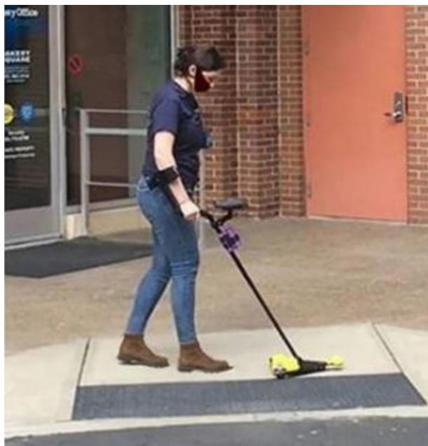
A technician uses a curbMet© to collect curb ramp data.
